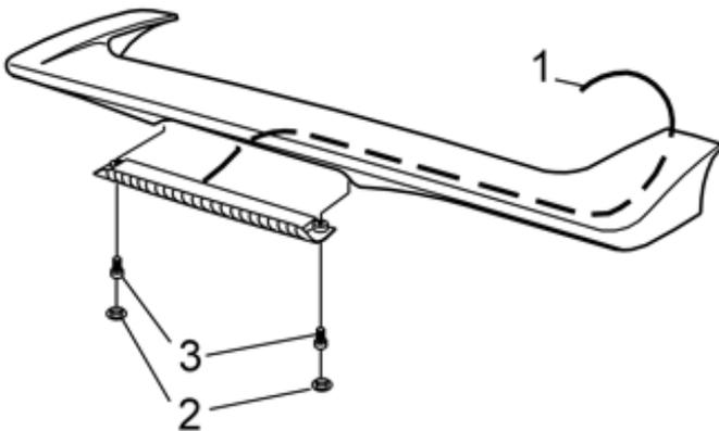
Route the cable (1) through the spoiler. Drill at the brake lamp. Thread a piece of wire or a thin plastic rod into the hole for the cable lead-in. Then tape the terminal and the cable to the wire and pull it out through the hole.
