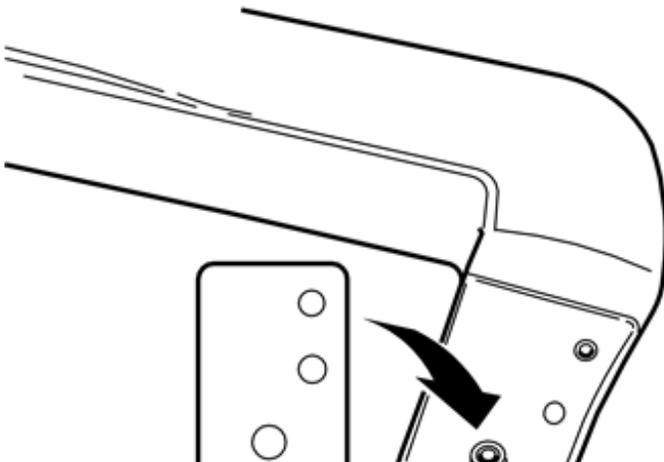
Position the tape on the mating surfaces. Press the tape into place. Leave the thick outer protective film in place.
