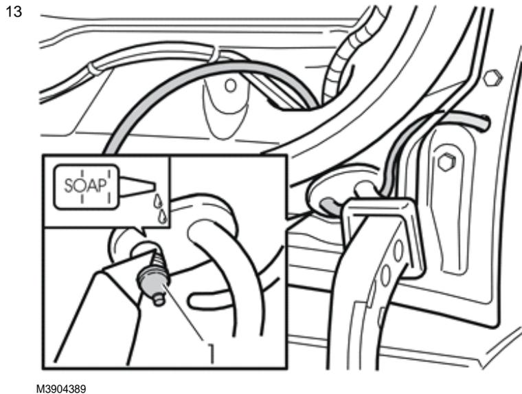
Cut the rubber nipple (1) off the rubber grommet for the brake lamp. Do not damage the existing washer hose
